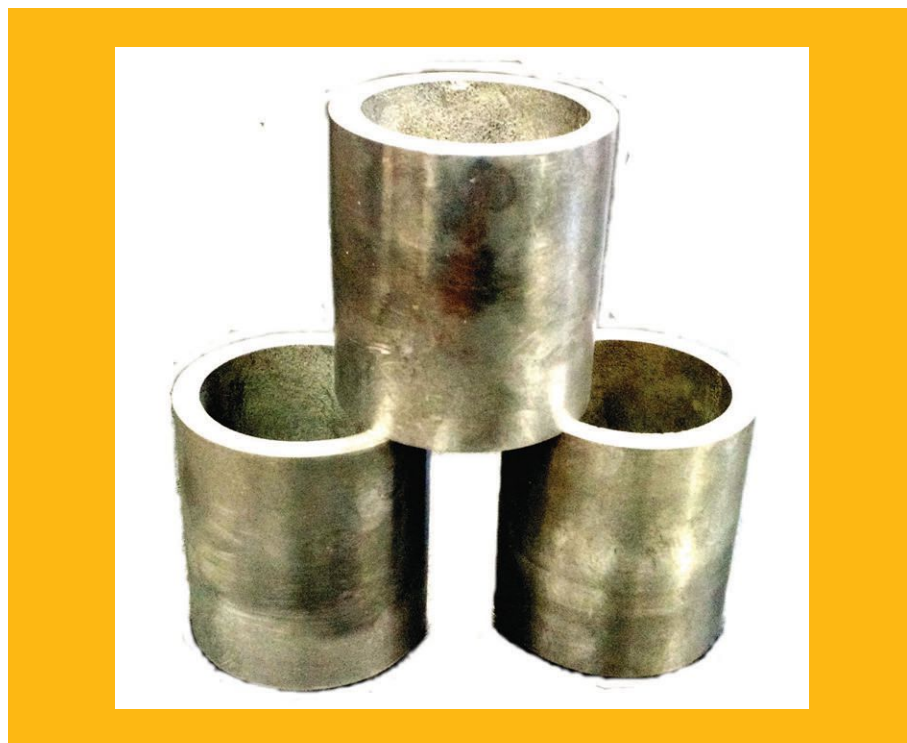
Figure 1 | Lightweight self-lubricating metal matrix composites represent a new approach for potentially improving automobile fuel efficiency. (Figure courtesy of Intelligent Composites, LLC.)
